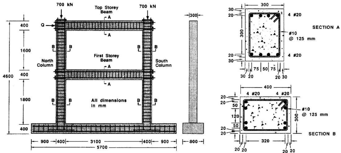
Figure 5.17: Two story RC frame: geometry and reinforcement details (Vecchio and Emara 1992).
