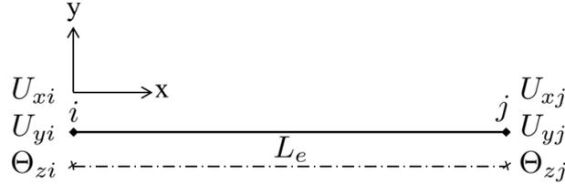
Figure 3.7: 2-node finite element Timoshenko beam
