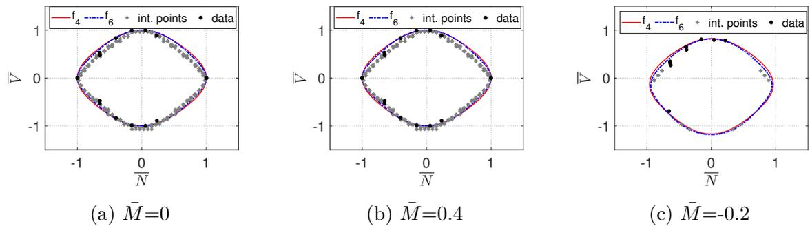
Figure 5.50: M2 section: Axial force - shear force interaction diagrams obtained by polynomials  $f_4$ ,  $f_6$  compared to data by numerical simulations and interpolated points.
