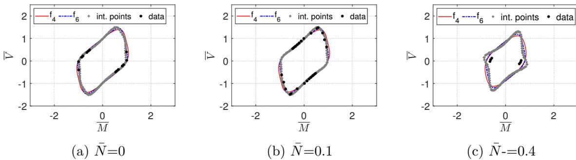
Figure 5.52: M4 section: Moment - shear force interaction diagrams obtained by polynomials  $f_4$ ,  $f_6$  compared to data by numerical simulations and interpolated points.
