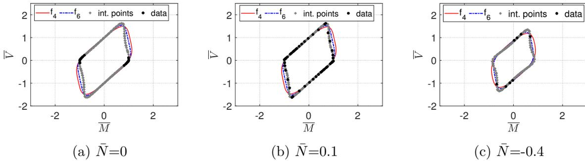
Figure 5.46: M1 section: Moment - shear force interaction diagrams obtained by polynomials  $f_4$ ,  $f_6$  compared to data by numerical simulations and interpolated points.
