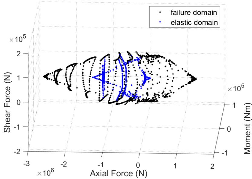
Figure 2.35: Interaction diagrams (discrete points) for M3 section (initial validated model: 1<sup>st</sup> characteristic state (‘elastic domain’) and 3<sup>d</sup> characteristic state (‘failure’).
