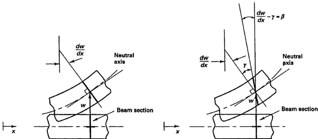
Figure 1.17: Kinematic assumptions for (a) Euler-Bernoulli and (b) Timoshenko beam (Bathe 2006).
