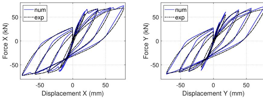
(a) Force-displacement, X direction (b) Force-displacement, Y direction
