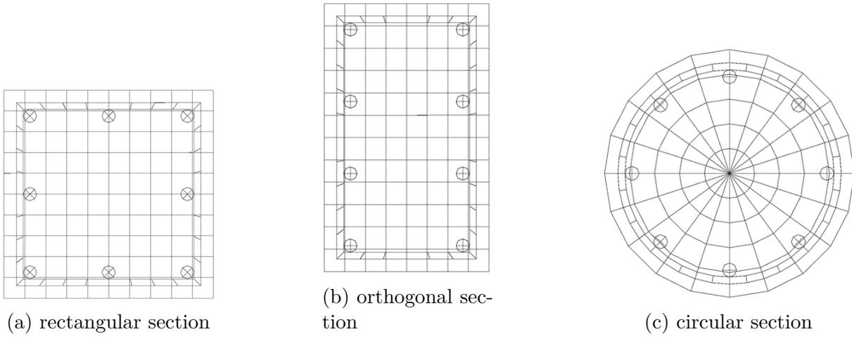
Figure 2.37: Different sections of equal areas and reinforcing ratios.
