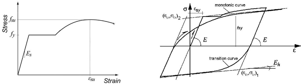
(a) Uniaxial steel behavior under monotonic loading. Modified Figure: its original version is found in Kunnath et al. 2009
