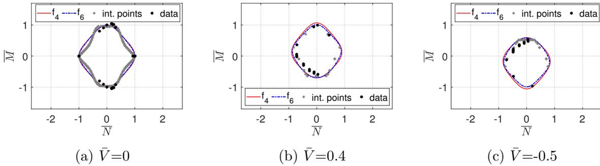
Figure 5.51: M4 section: Moment - axial force interaction diagrams obtained by polynomials  $f_4$ ,  $f_6$  compared to data by numerical simulations and interpolated points.
