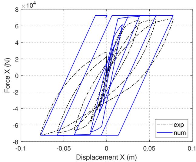
Figure 5.7: RC cantilever column S1: Numerical (1<sup>st</sup> approach) vs. experimental global response (cyclic loading of alternate sign).
