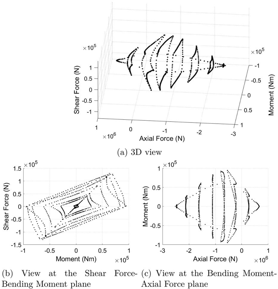
Figure 2.26: 2<sup>nd</sup> characteristic state (elastic domain of steel rebars): Interaction diagram (discrete points) obtained by numerical simulations.
