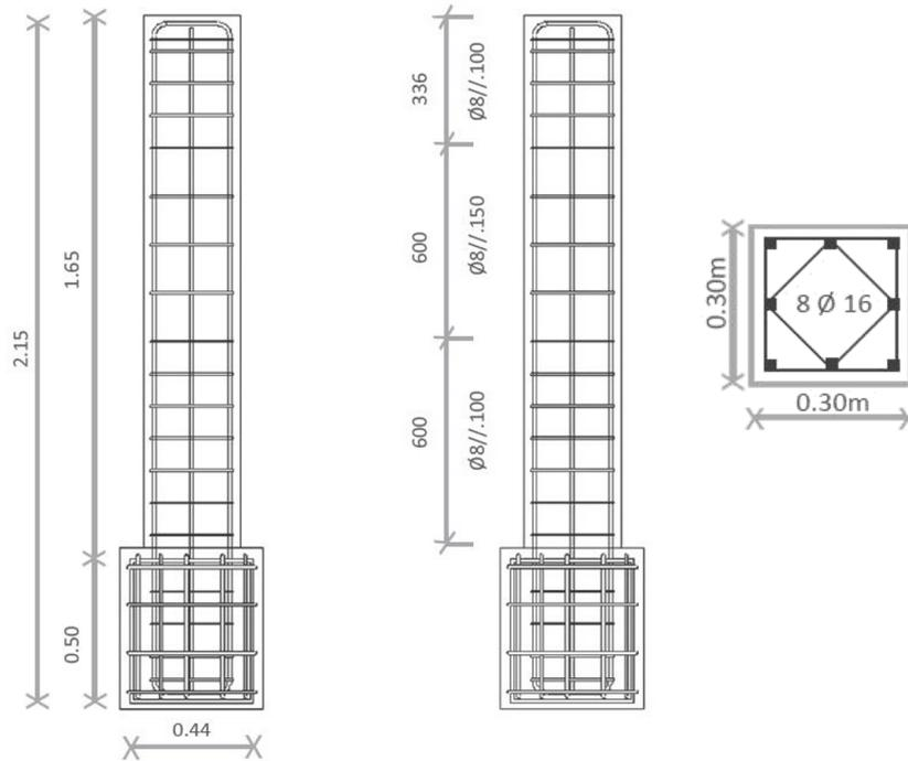
Figure 5.10: RC cantilever column (carbon steel): Specimen dimensions (left), shear reinforcement details (center) and cross-section of the specimen (right).
