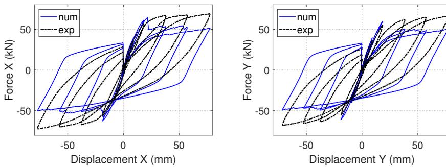
(b) Force-displacement, X direction (c) Force-displacement, Y direction
