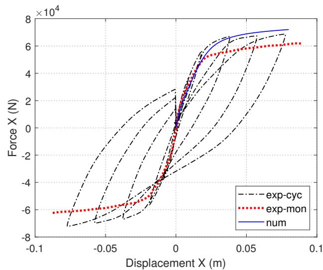
Figure 5.5: RC cantilever column S1: Numerical vs. experimental global response (monotonic loading).
