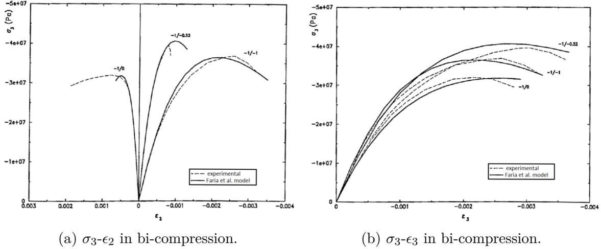
Figure 2.2: Comparisons of the numerical predictions (Faria 1994) with experimental results (Kupfer et al. 1969) for concrete under bi-compression ( $\sigma_1 = 0$ ) for  $\sigma_3/\sigma_2 = -1/0$ ,  $\sigma_3/\sigma_2 = -1/-1$  and  $\sigma_3/\sigma_2 = -1/-0.52$ .
