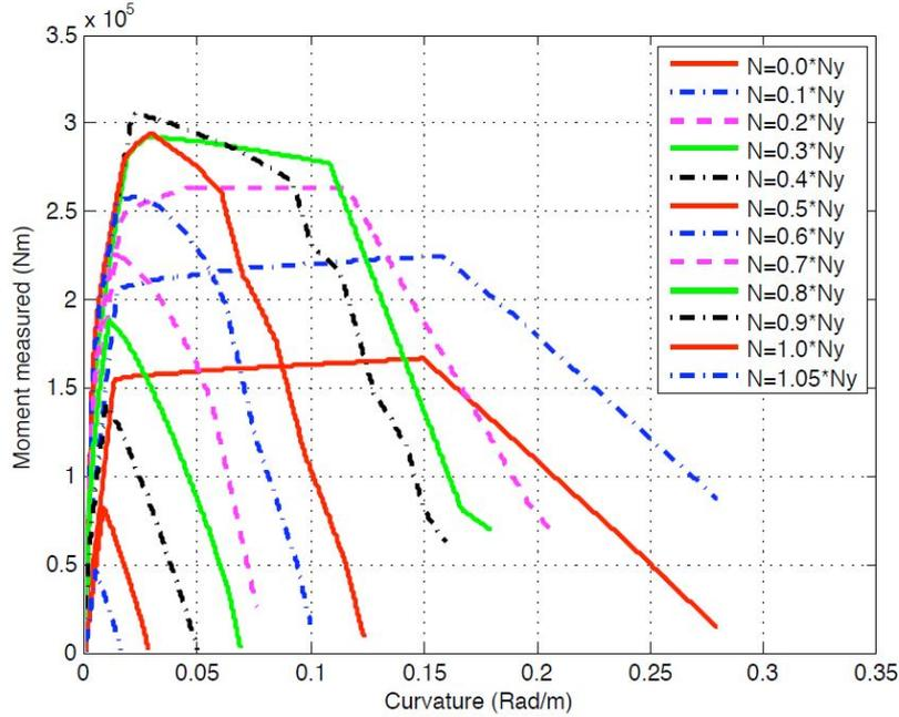
Figure 4.6: Moment-curvature relations for different levels of axial force, obtained by enhanced multi-fiber beam calculations (Pham et al. 2010).
