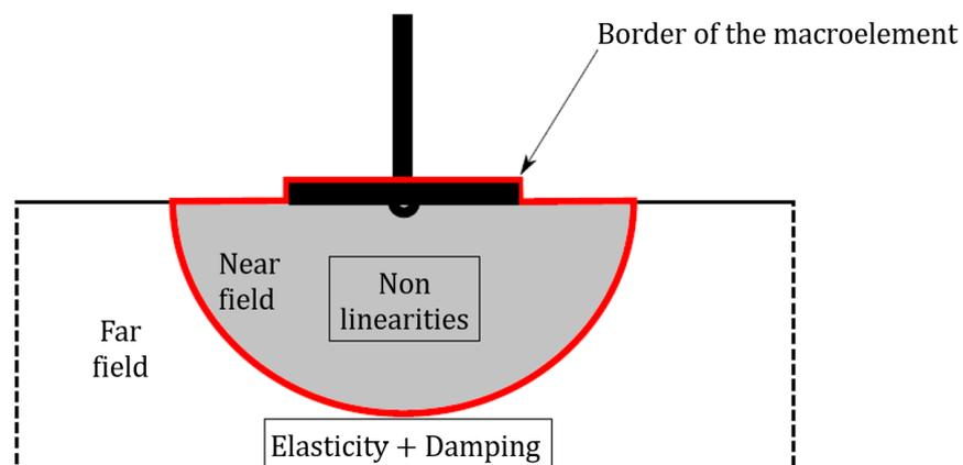
Figure 3.1: The macroelement concept for SSI problems (Grange 2008).
