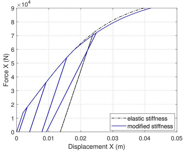
Figure 3.10: Comparison of the global responses of a cantilever beam subjected to a cyclic transversal load, using the elastic stiffness and the modified (steel) stiffness.
