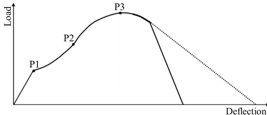
Figure 1.12: Typical load-deflection relationship for reinforced concrete elements.
