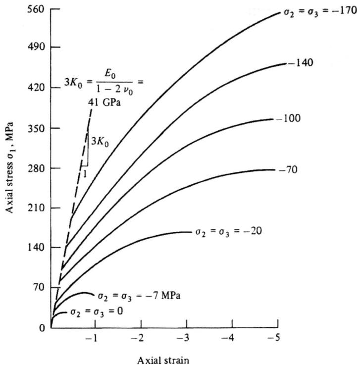
Figure 1.4: Triaxial stress-strain relationship for concrete (Balmer 1949).
