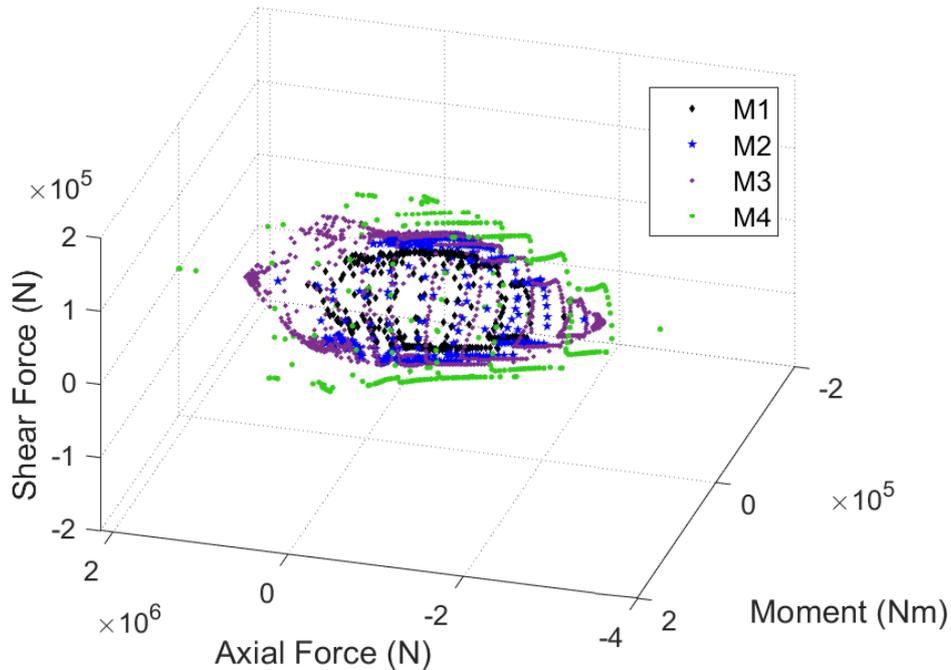
Figure 2.28: 3<sup>d</sup> characteristic state ('failure'): Interaction diagrams (discrete points) for sections with different reinforcement ratios obtained by numerical simulations (M1 (1.01%), M2 (2.01%), M3 (initial validated model, 2.57%) and M4 (5.15%).
