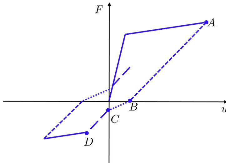
Figure 3.12: Schematic representation of cyclic response by considering a simplified approach for stiffness degradation, the pinching effect and stiffness recovery.
