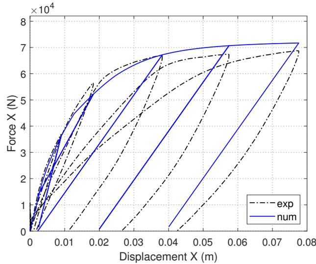
Figure 5.6: RC cantilever column S1: Numerical vs. experimental global response (cyclic loading of constant sign).
