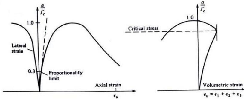
Figure 1.3: Concrete behavior during compression (Chen 2007).
