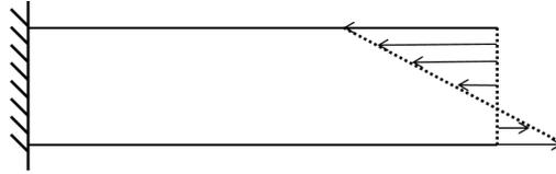
Figure 2.22: 2D radial test: coupled bending - axial loading.
