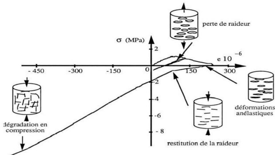
Figure 1.5: Uniaxial concrete behavior under cyclic loading (Ramtani 1990).
