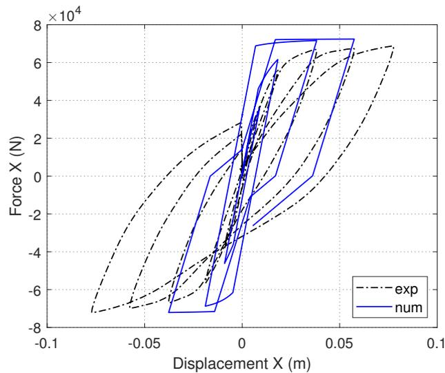
Figure 5.9: RC cantilever column S1: Numerical (calibrated  $2^{nd}$  approach) vs. experimental global response (cyclic loading of alternate sign).
