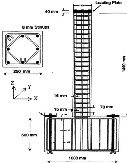
Figure 2.5: RC columns: geometry (Gutierrez et al. 1993).
