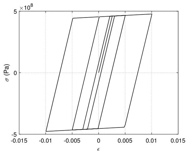
Figure 2.4: Steel cyclic behavior during 1D cyclic test.
