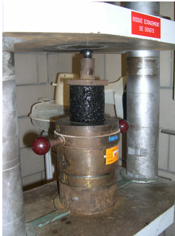
FIGURE 1.31: Essai Duriez (base documentaire IFSTTAR/MAST/MIT)
