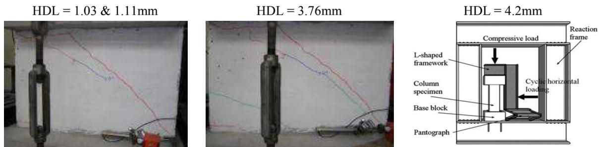
Figure. A-10: Crack pattern of the reference short wall VC1
