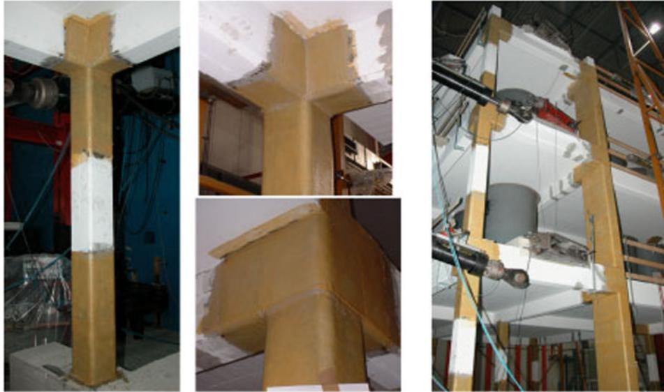
Figure 4-15: SPEAR-Configuration de renforcement (Di Ludovico et al. 2008)
