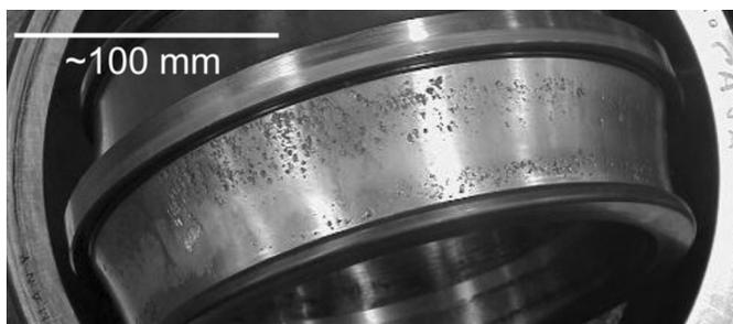
RCF of inner raceway of spherical roller bearing [OLV 05]
