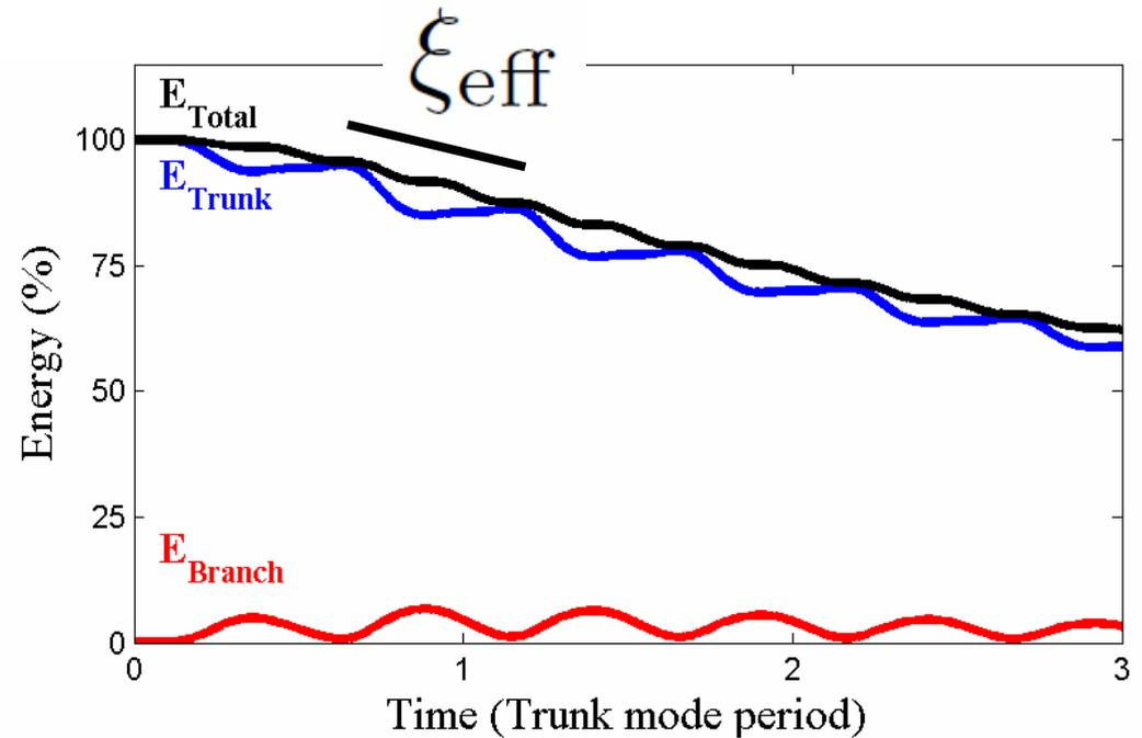
The structure is **effectively damped**
