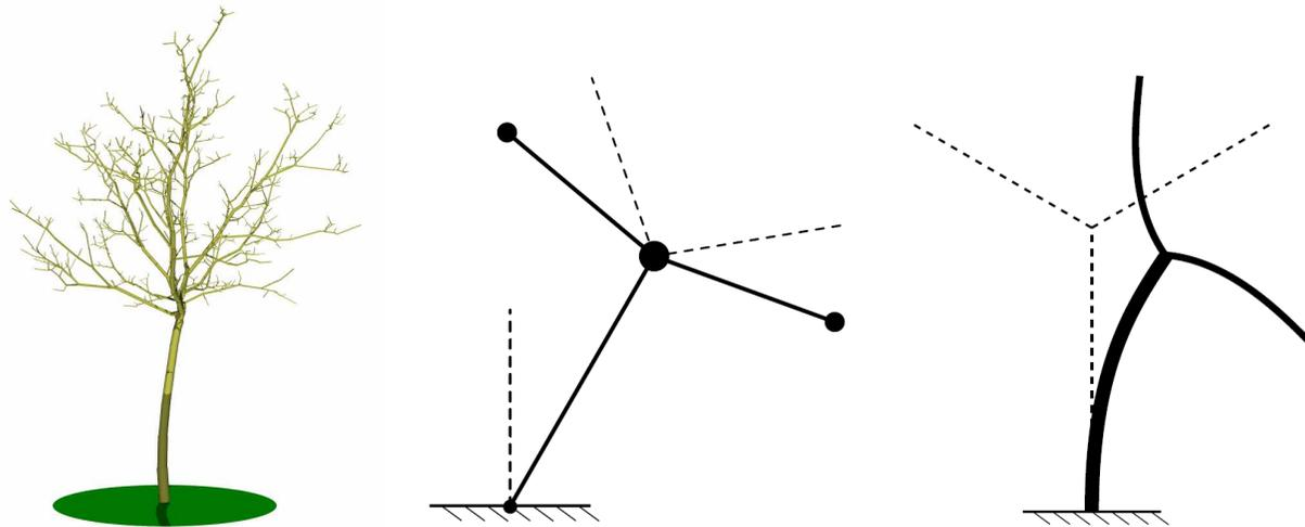
A robust bio-inspired mechanism to damp large-amplitude motions
