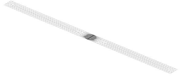
Fig. 3. CAST3M model used for the infinite straight tape computations.
