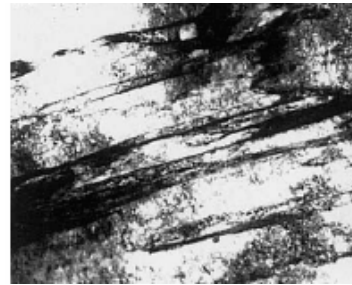
Martensite obtained by quenching after austenisation at 1050°C
