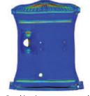
Cracking in a pre-stressed concrete containment vessel
