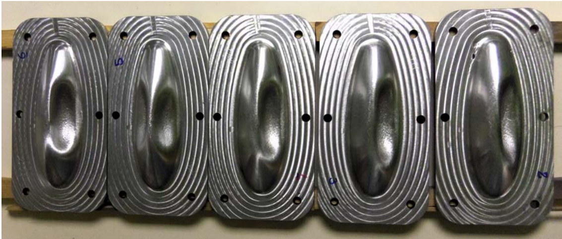
Figure 5.21: Deformed specimens after buckling; from left to right: specimen O/006, O/005, O/004, O/003 and O/002
